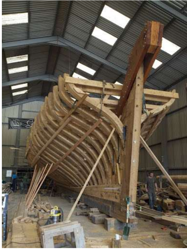
Assembling the ribs
