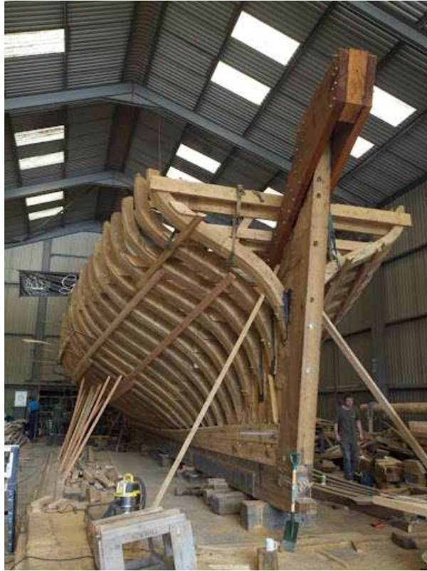
Assembling the ribs
