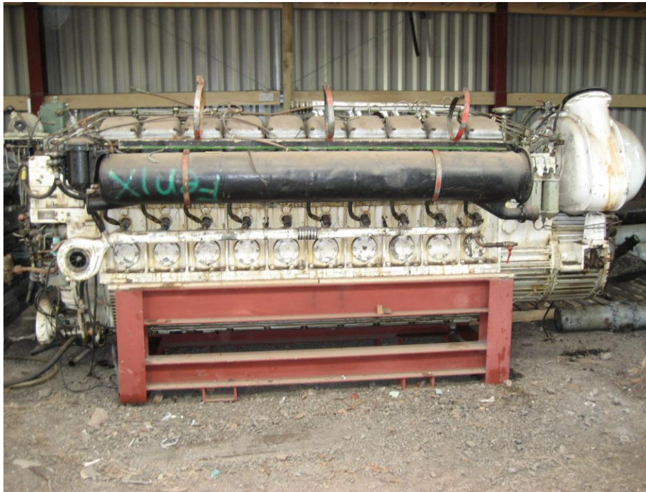
This Picture shows one of the original MB511 V-20 cylinder diesel engines.
